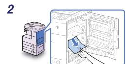
Remove any jammed paper protruding from the lower part of the fixing unit.
